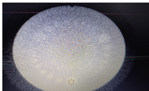
Fig. 4 The contrast-to-noise ratio (CRN) measured into the selected region of interest (ROI)
