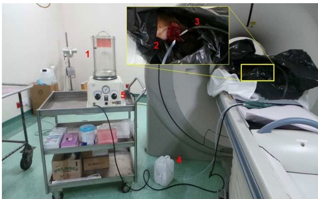
Fig. 2 The whole modified PMCTA system was used in our center. The embalming machine was used to inject a mixture of nonionic, water-soluble contrast medium and PEG 200 (no. 1). The inlet and outlet catheters cannulated into the right CCA (for arterial & dynamic phases) and IJV (for venous phase) labeled as no. 2 & 3. Outlet collection container placed on the floor (no. 4) with collection tube attached to the catheters. No. 5 is the pressure and infusion rate regulator and gauge on the embalming machine which controlled the pressure and infusion rate manually during infusion
